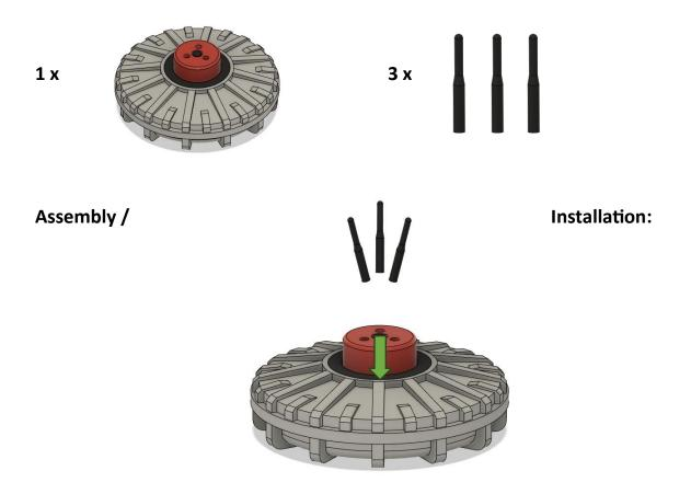
To assemble the model, put the 3 antennas inside the 3 holes on the top of the red tower as shown in the picture above (See green arrow). Optional: apply a drop of glue in the hole before inserting the antenna.
